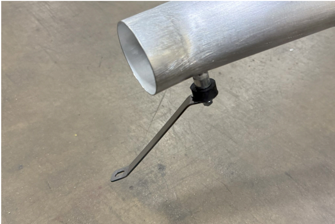
15. Mount the provided Z bracket onto the rubber vibration mount using the provided M6 nut and washer.
