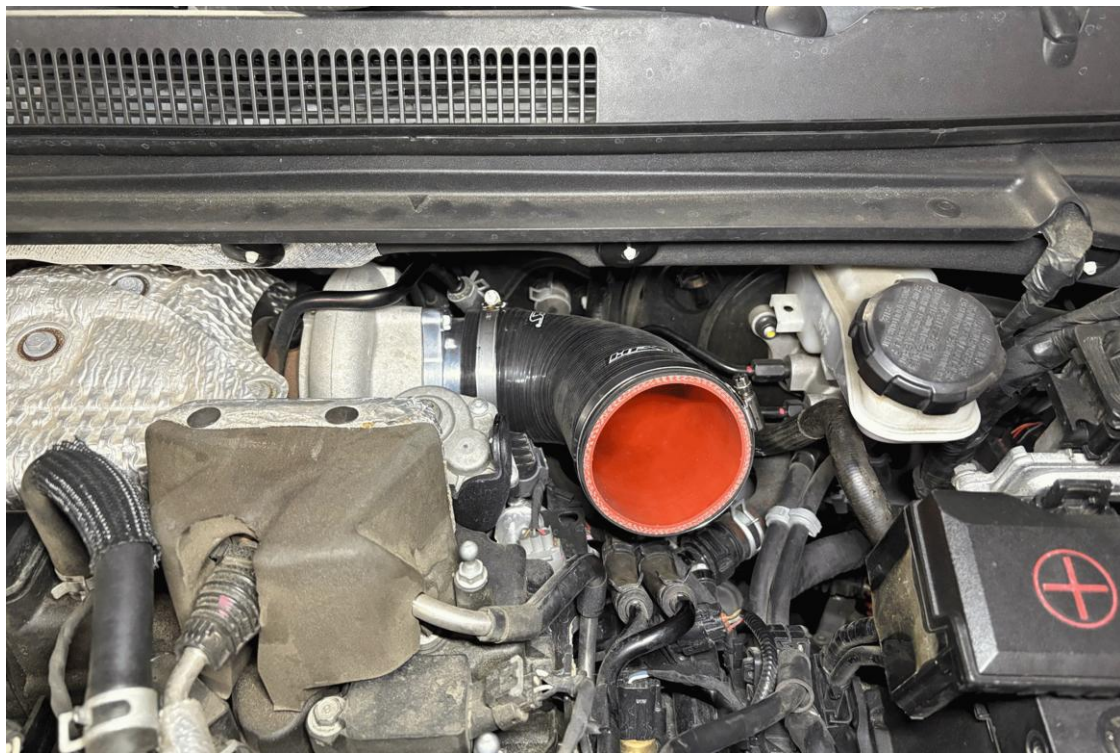
10. Loosely connect the HPS elbow coupler, along with the provided hose clamps, onto the turbo inlet.
